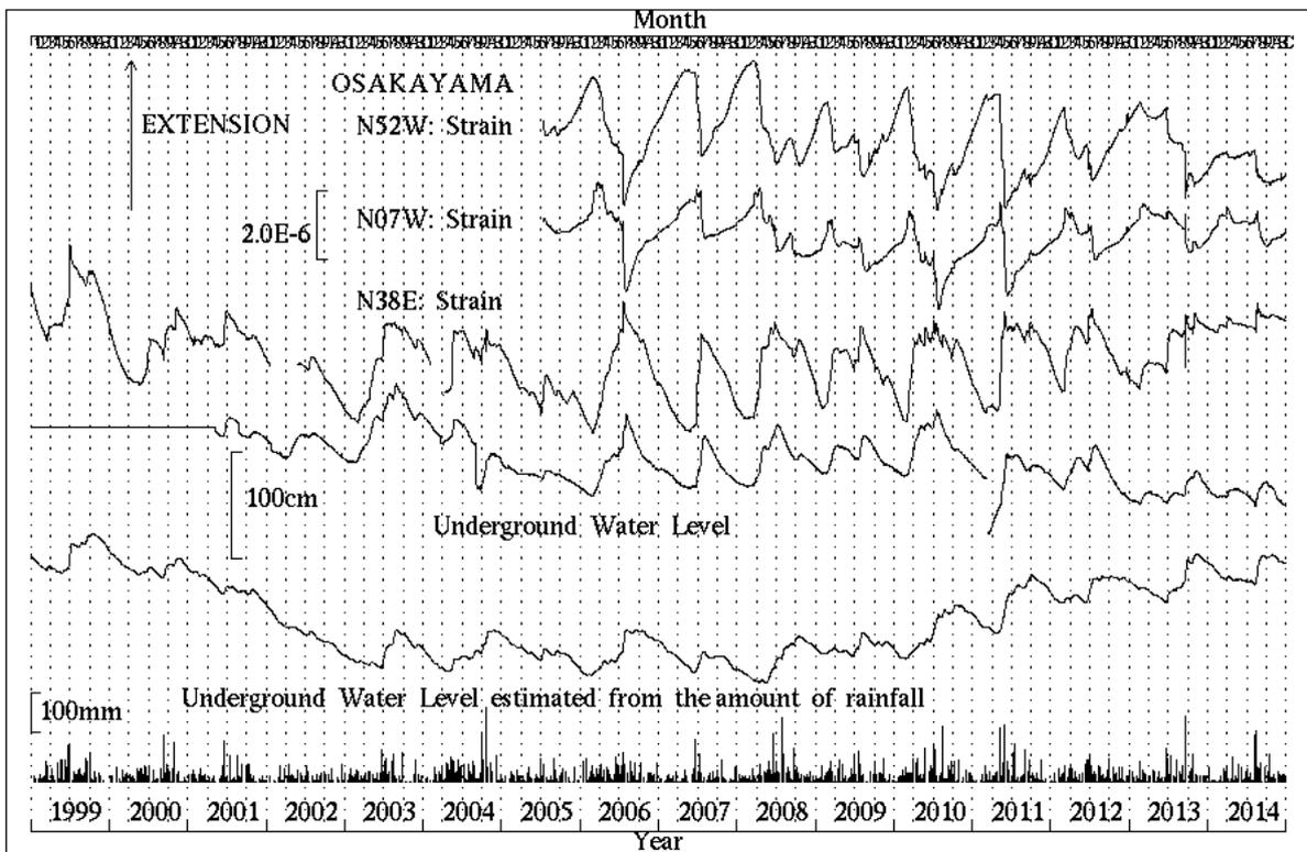
Fig.3 Changes of the strain rate observed at Osakayama observatory.
