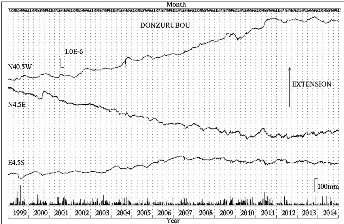
Fig.2 Changes of the strain rate observed at Donzurubou observatory.
