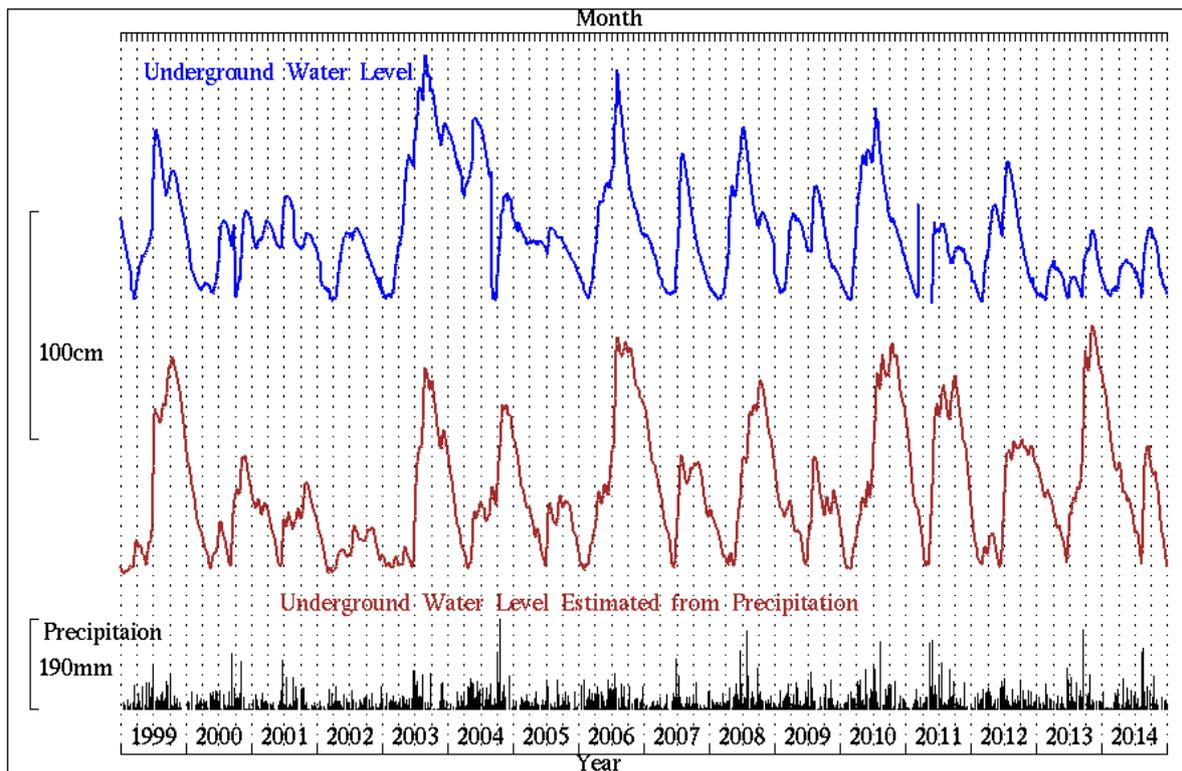
Fig.6 The underground water level at the Osakayama observatory. Upper shows the actual measurement. Lower shows the estimated value from the precipitation.
