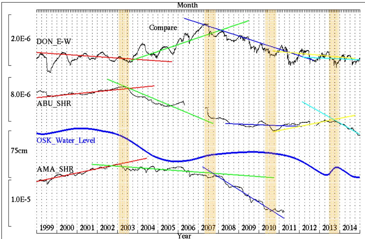
Fig.5 Comparison of strain rates among Donzurubou, Abuyama and Amagase observatories. Ground water level recorded at Osakayama observatory is shown for the reference.
