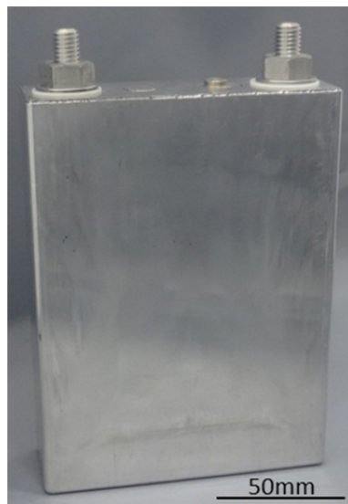
Fig. 6-1 Appearance of a 27 Ah HC/Na[FSA]-[C 3 C 1 pyrr][FSA]/NaCrO 2 prismatic cell. External size: 113×150×38 mm. Weight: 1.08 kg.
