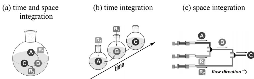
**Figure 2.** Classification of integrated synthesis. A: Starting material, B: intermediate, C: product, R<sub>1</sub> and R<sub>2</sub>: reagents.
