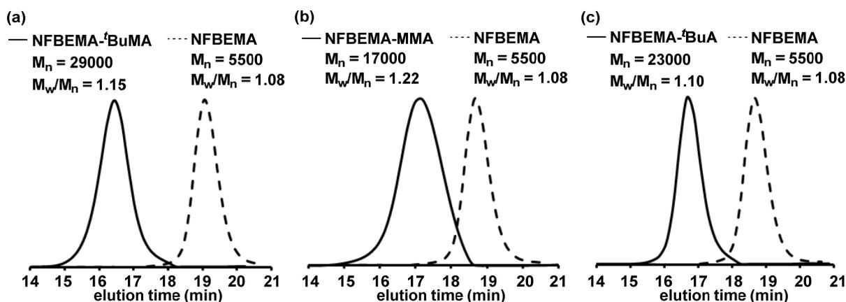
**Figure 3.** Size exclusion chromatography traces of block copolymers obtained in the integrated flow microreactor system. (a) 2-(Nonafluorobutyl) ethyl methacrylate (NFBEMA) ( $-40$  °C)–*tert*-butyl methacrylate (*t*BuMA) ( $20$  °C), (b) 2-(nonafluorobutyl)ethyl methacrylate (NFBEMA) ( $-40$  °C) – methyl methacrylate (MMA) ( $-30$  °C), and (c) 2-(nonafluorobutyl)ethyl methacrylate (NFBEMA) ( $-40$  °C) – *tert*-butyl acrylate (*t*BuA) ( $-20$  °C)
