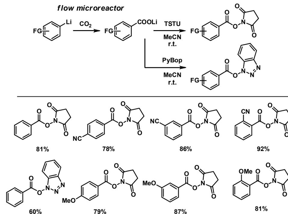
**Figure 1.** Flow microreactor synthesis of active esters.
