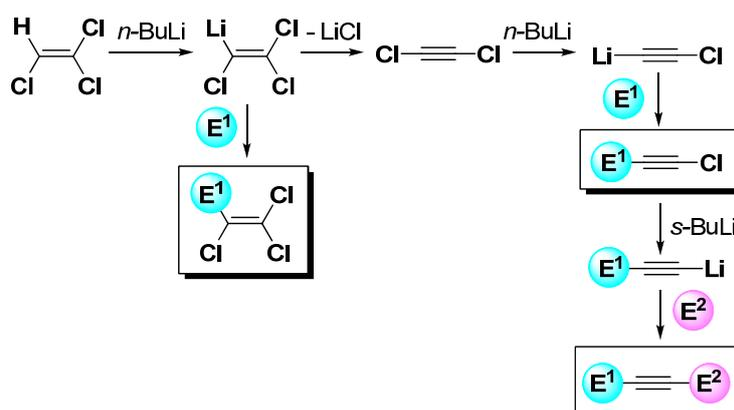
**Figure 1.** Synthesis of chloroalkenes and alkynes from trichloroethene.
