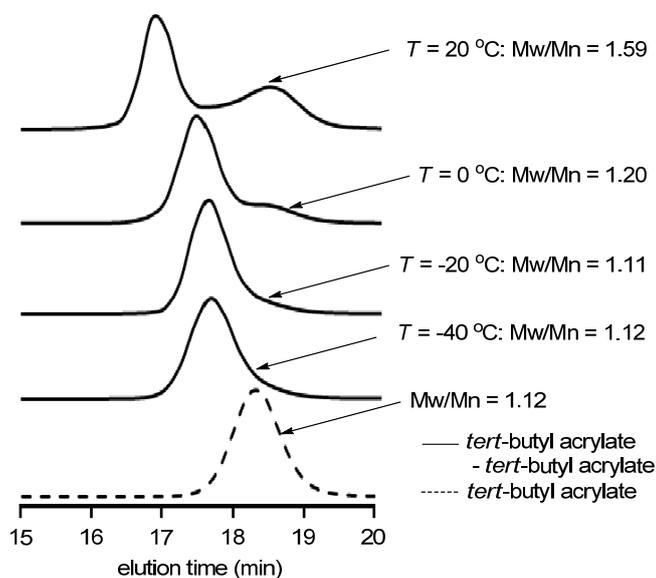
**Figure 2.** Size exclusion chromatography traces of sequential anionic polymerization of *tert*-butyl acrylate in the integrated flow microreactor system. Effect of reaction temperature ( $T$ ) in  $t^{R2}=2.24$  s.
