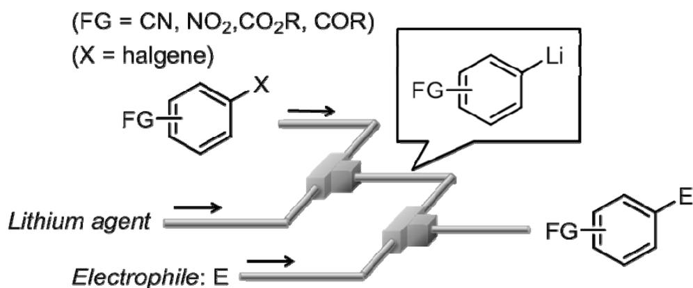
**Figure 1.** Generation of aryllithiums bearing electrophilic functional groups and their reactions with electrophiles using a flow microreactor system
