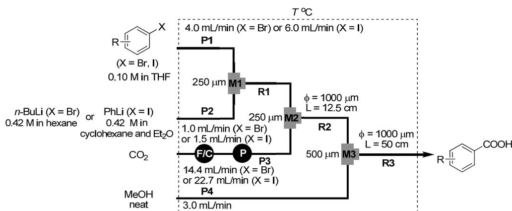
**Scheme 1.** A flow microreactor system for the reactions of aryllithiums with CO<sub>2</sub> gas. T-shaped micromixers: **M1**, **M2**, **M3**; microtube reactors: **R1**, **R2**, **R3**; flow controller: FC; pressure gage: P.
