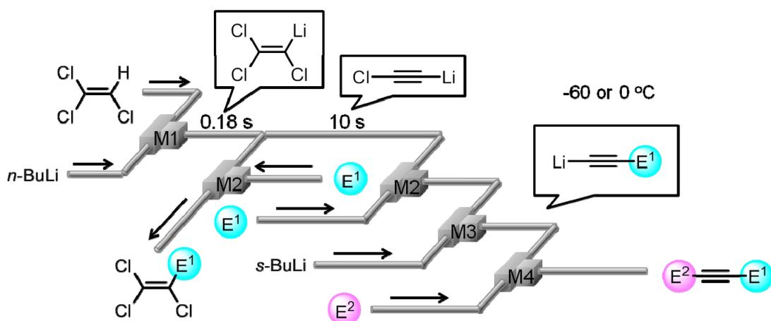
**Figure 4.** Selective synthesis of alkenes and alkynes by switching of the reaction-pathways of trichlorovinyl lithium based on the residence time control.
