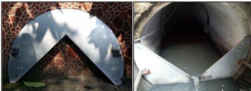
Figure 4-2 A 90°V-Notch weir
