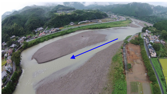
Photo 3 Aerial picture of changed water route due to flood of Typhoon No.11, 2015.
