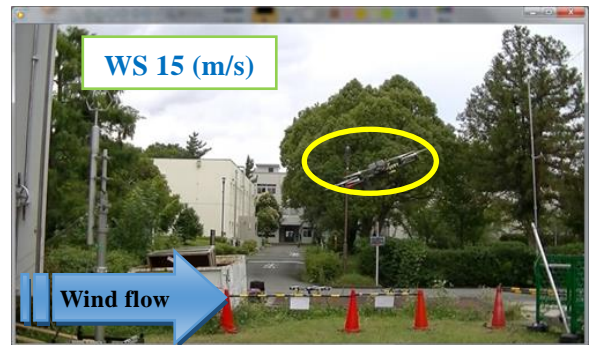
Fig . 7 Screen capture of drone stability at wind speed 5 m/s, 10 m/s and 15 m/s
