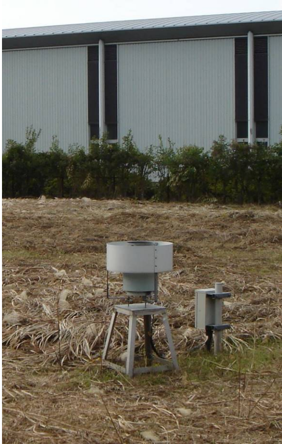
Photo 4 Tipping bucket rain gauge in the field
