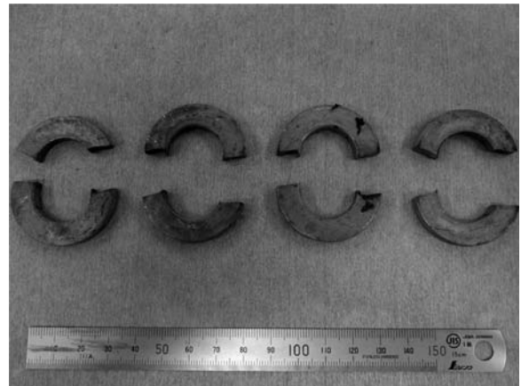
Fig. 3. Four metallic washers which were removed.
