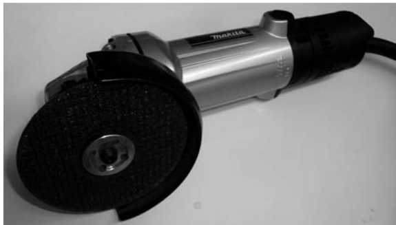
Fig. 2. The electric grinder used to cut the washers.
