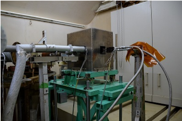
Fig.1 New neutron source installed in KURRI-LINAC
