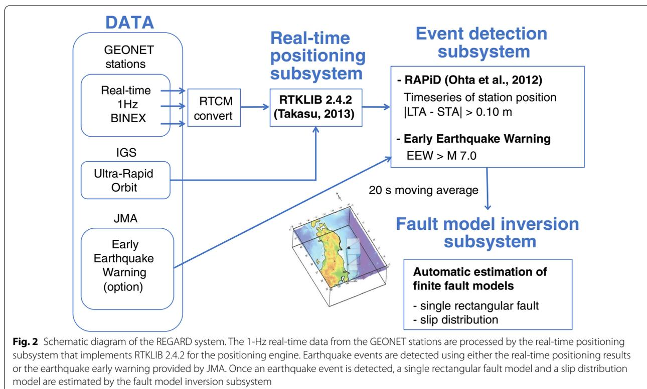
**Fig. 2** Schematic diagram of the REGARD system. The 1-Hz real-time data from the GEONET stations are processed by the real-time positioning subsystem that implements RTKLIB 2.4.2 for the positioning engine. Earthquake events are detected using either the real-time positioning results or the earthquake early warning provided by JMA. Once an earthquake event is detected, a single rectangular fault model and a slip distribution model are estimated by the fault model inversion subsystem
