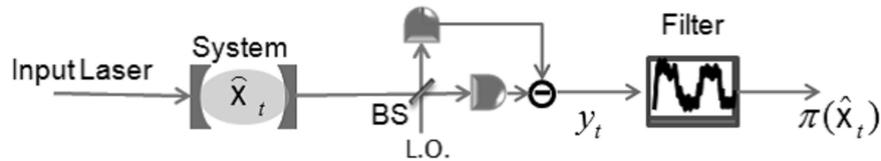
Fig. 1 Schematic of the quantum Kalman filter. First, the system couples with a input laser. The output laser is mixed, by a beam splitter(BS), with a strong reference light called the local oscillator(LO), and two outputs are then respectively detected via a photon detector. This whole measurement configuration is called the homodyne detection. Finally, the quantum Kalman filter uses the output to calculate the best estimation  $\pi(\hat{x}_t)$ .
