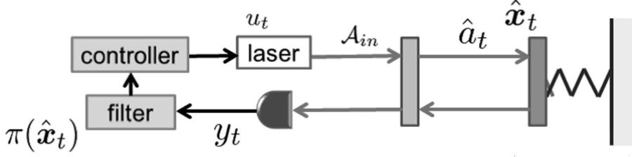
Fig. 2 Schematic of the optomechanical oscillator. The right end mirror of the Fabry-Perot cavity serves as the oscillator, where  $\hat{\mathbf{x}}_t$  is the system variable,  $\hat{a}_t$  is an annihilation operator corresponding to the intra-cavity, and  $\mathcal{A}_{in}$  is the mean amplitude of the input laser.
