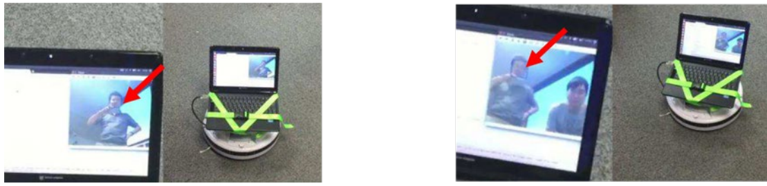
Fig. 3. Robot and captured image. Left: a situation with a single person in the robot's field of view. Right: a situation with two persons in the same field. Detected faces are indicated with red arrows.
