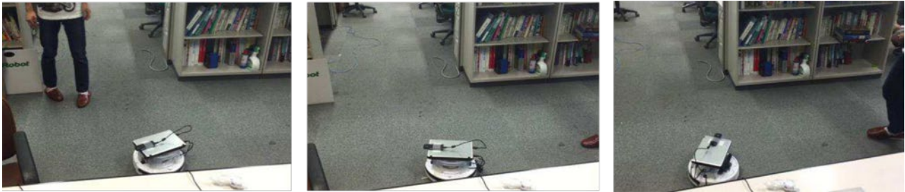
Fig. 4. Robot and captured image. Left: the robot detects the person in front of it. Middle: the robot fails to detect the person using its main camera and instead detects moving object with its omnidirectional camera. Right: the robot rotates toward the person.
