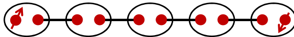
Figure 1.9: Illustration of the AKLT state for spin-1 chains. Each red ball expresses a spin-1/2 degrees of freedom. The solid line indicates a singlet state between neighboring spins. The solid circle denotes a symmetrization operation of the wavefunction for recovering the state expressed in terms of the original spin-1 degrees of freedom.
