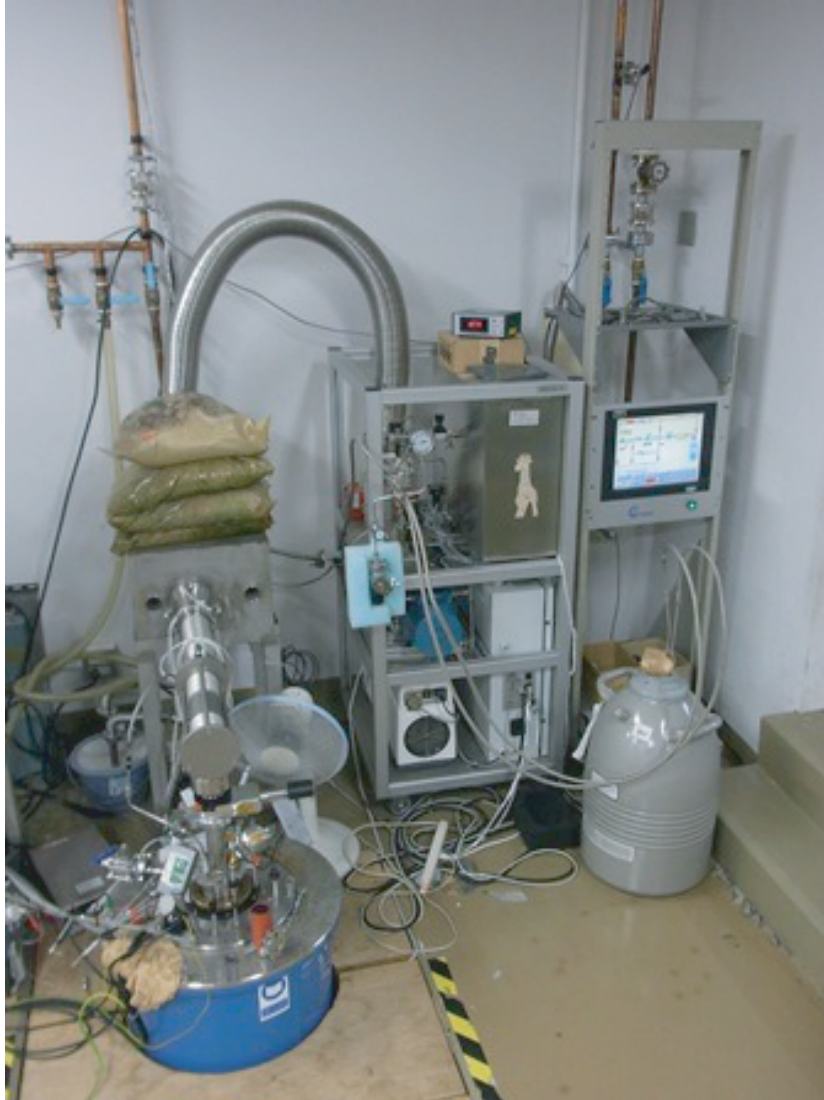
Figure 3.1: Picture of the measurement system with a gas handling system and superconducting magnet. The 12-14 T solenoidal superconducting magnet is placed under the floor. We operated the system by using a touch panel. In order to reduce vibration noise from the vacuum pumps, which may cause heating, we set up an anti-vibration block with several sandbags between the cryostat and the gas handling system.
