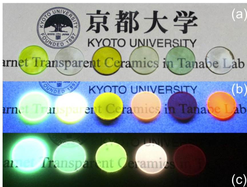
Figure 2.8. Garnet transparent ceramic persistent phosphors prepared in Tanabe Lab (a) under fluorescent lamp (b) under UV (254 nm) lamp (c) in the dark; samples from left to right: \text{Y}_3\text{Al}_2\text{Ga}_3\text{O}_{12}(\text{YAGG}):\text{Ce-Cr} (chapter 3), \text{Y}_3\text{Al}_2\text{Ga}_3\text{O}_{12}(\text{YAGG}):\text{Tb-Cr} (chapter 4), \text{Gd}_3\text{Al}_2\text{Ga}_3\text{O}_{12}(\text{GAGG}):\text{Ce-Cr} , \text{Y}_3\text{Al}_2\text{Ga}_3\text{O}_{12}(\text{YAGG}):\text{Pr-Cr} (chapter 4), \text{Y}_3\text{Al}_2\text{Ga}_3\text{O}_{12}(\text{YAGG}):\text{Cr} (chapter 5), \text{Gd}_3\text{Ga}_5\text{O}_{12}(\text{GGG}):\text{Cr-Eu} (chapter 6)
