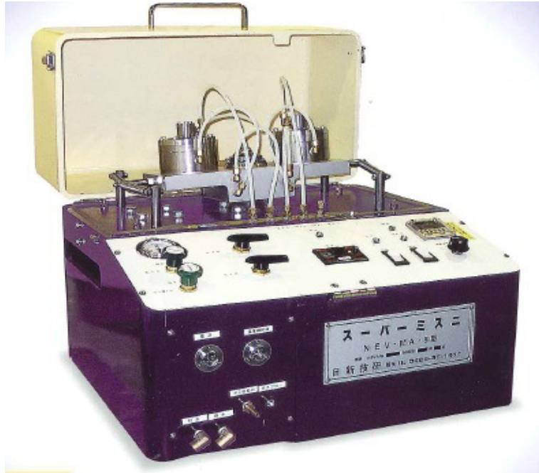
Fig. 2.1. Picture of a vibratory ball mill used for this thesis.
