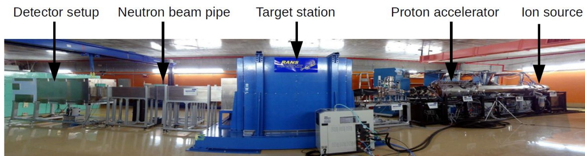
Figure 1. Entire view of RANS. This is about 15 m in total length, consists of an ion source, a proton accelerator, a target station, a neutron beam pipe and a camera box.
