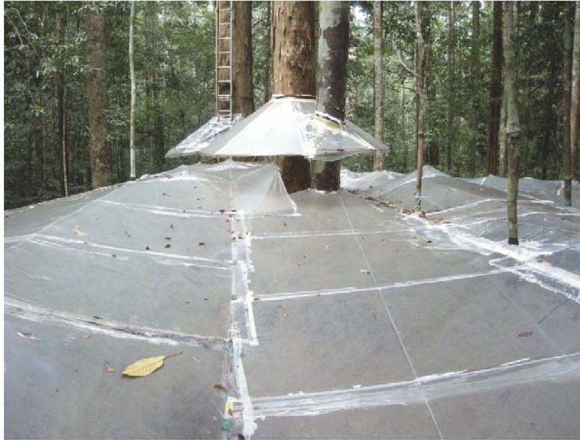
Fig. 4 Big umbrella set for the experiment to artificially cause drought for a target tree.
