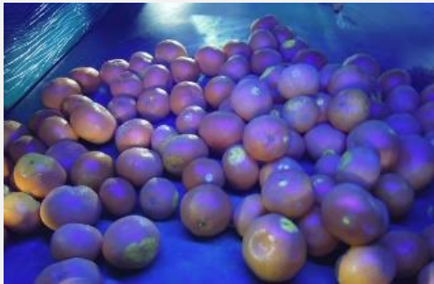
生傷、腐敗の検出 / Pinhole and rotten fruit detection for separation from healthy fruits
