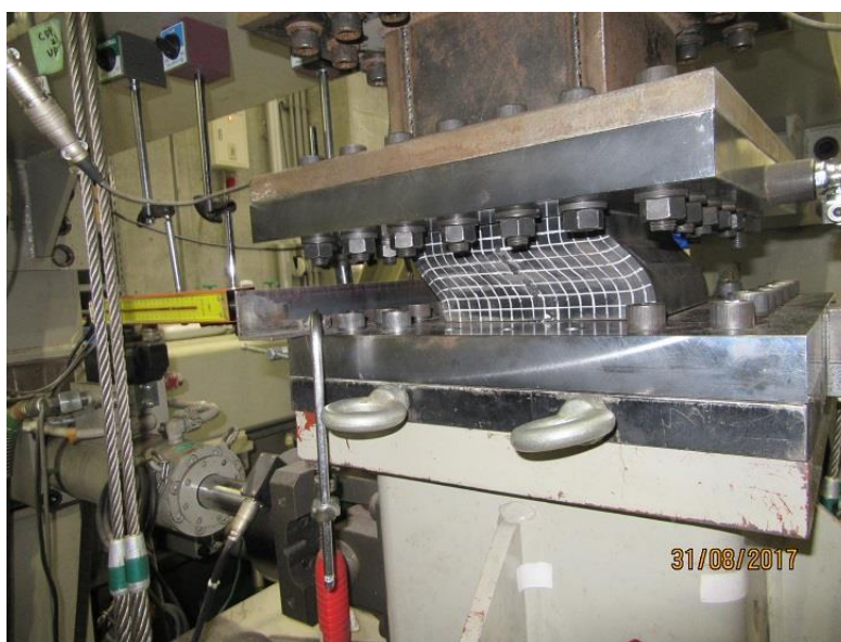
Figure 6.5: Bearing Specimen (No. 1214) being pushed to 36.75 mm displacement.
