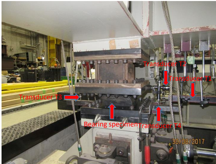
Figure 6.4: Displacement transducers attached to the specimen.
