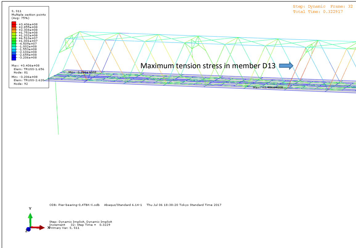
Figure 7.12: Maximum stresses with elastomeric bearings due to 0.4g Thabeikkyin Earthquake in X-direction.
