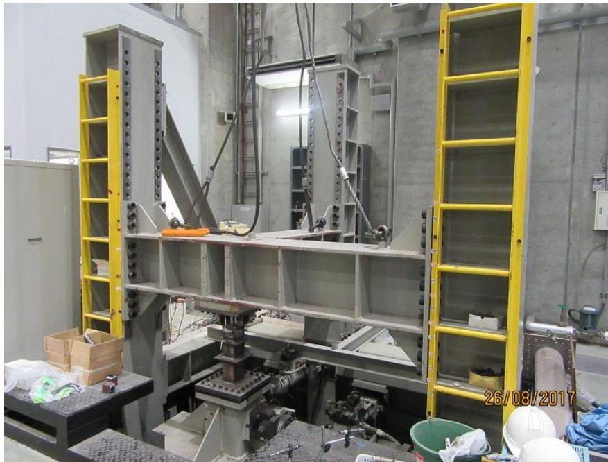
Figure 6.2: Six DOF universal testing machine in Structural Engineering Laboratory.
