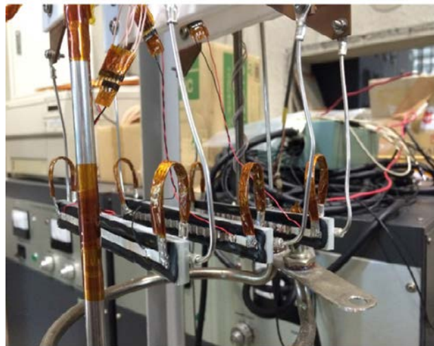
Fig. 1. Photo of the test superconducting tapes with and without fins.
