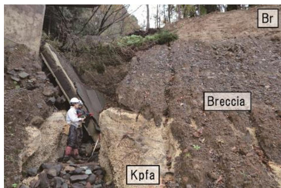
Fig. 36 Stratigraphic succession observed at landslide NGN-3. The white layer in the bottom is Kpfa, which is overlain by breccia layer consisting of obsidian and pumice grains. the landslide by erosion.
