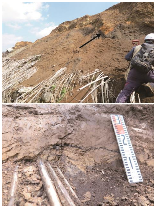
Fig. 26 Landslide AVL-4 (upper) and the contact between the original ground surface and the debris (lower). We see grass stems beneath the debris. surface of Br with lava blocks was widely exposed.
