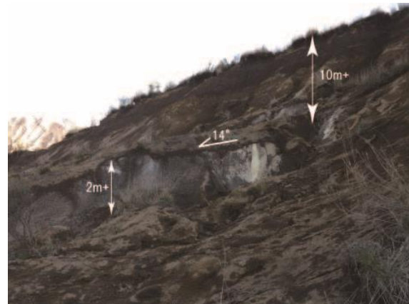
Fig. 34 A sliding surface formed in white Kpfa (EBS-W5). The sliding surface dips 14° to the left.
