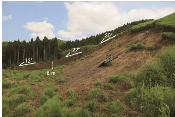
Fig. 25 Oblique view of landslide AVL-3. Surface slope angles changed from 30° in higher elevations to 12° in lower. A sliding surface of Br with lava blocks was widely exposed.
