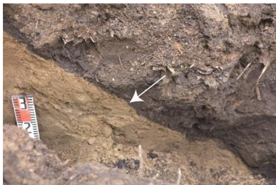
Fig. 21 A sliding surface formed in the Br layer covered by debris, which was observed at the bottom of the head scarp (SWT-3).
