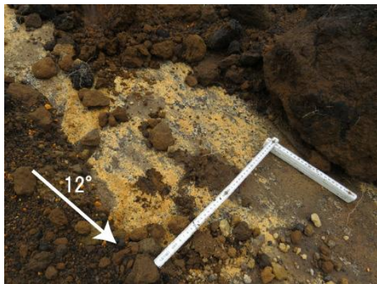
Fig. 23 An exposed sliding surface at the base of Kpfa (white), which occurs in patches on the underlying B1Br in AVL-1.
