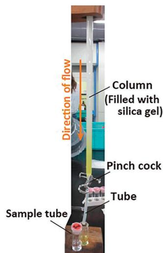
Fig. 2. Equipment used for column chromatography.
