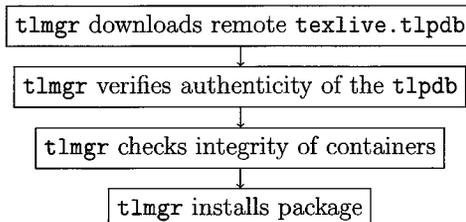
Checking authenticity of the downloaded `texlive.tlpdb` is done by first downloading its respective checksum `texlive.tlpdb.sha512`, as well as the cryptographic signature of the checksum file, named `texlive.tlpdb.sha512.asc`. The GNU Privacy Guard (`gnupg`) is used to verify that the downloaded signature and the checksum file agree. We refer the reader to introductions to asymmetric cryptography concerning details of this process.
