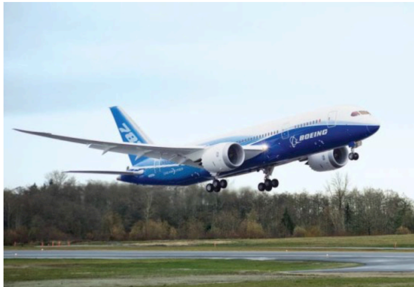
Fig. 1-7 The first flight of Boeing 787 – the world’s first wide-body passenger airplane applying composite to its primary structure. [1.20]
