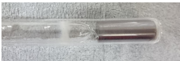
Figure 4.4: Tantalum crucible inside glass tube for synthesis of \text{Sr}_3\text{SnO} at 1200 °C.
