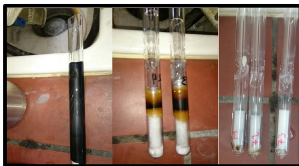
Figure 4.3: Silica tubes with \text{Sr}_{3-x}\text{SnO} samples synthesized in alumina crucibles under vacuum (left and middle pictures) showing varying evaporation of Sr. Synthesis with 0.3 atm argon pressure (right) shows almost no evaporation of Sr outside of crucible.
