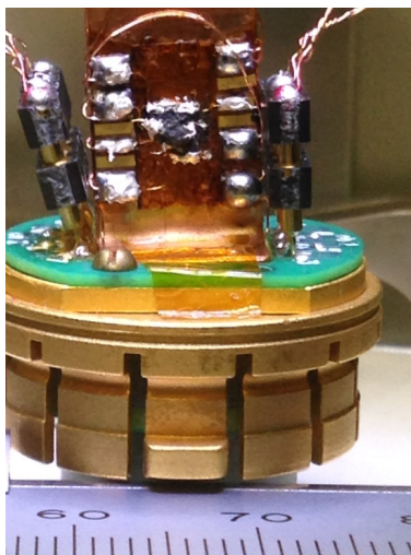
Figure 3.3: \text{Sr}_{3-x}\text{SnO} sample with five gold wires attached using silver epoxy for resistivity and Hall measurement using PPMS. Sample was covered with N-grease before moving the device from glovebox to PPMS.
