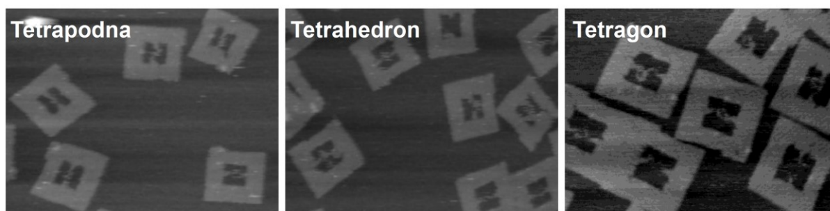
Figure 5. AFM images of tetrapodna, tetrahedron, and tetragon. The white rectangles with a window represent DNA origami frames.
