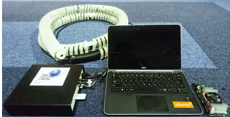
Figure 3.23: Hose-shaped rescue robot system including robot body (back), robot controller (left), laptop PC (middle), and embedded GPGPU board (right).
