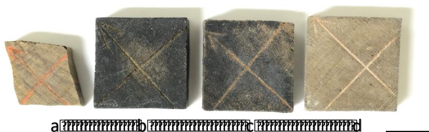
Fig. 4.7 Post-treatment appearance and coloration of the waterlogged Dysoxylum sp. wood after air drying: (a) untreated, (b) treated with PEG, (c) treated with trehalose, and (d) treated with keratin. The solid bar below represents 1 cm.
