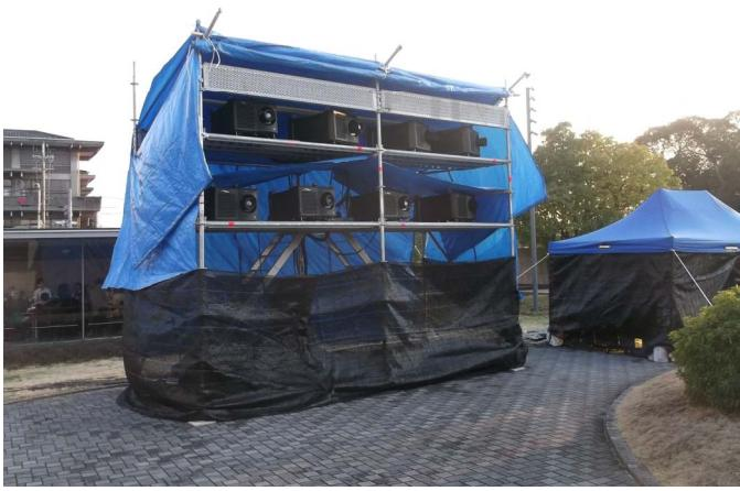
Fig. 10. Setting of eight projectors used for the projection onto the new building.
