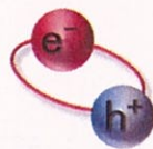
Figure 2.10 Exciton: electron-hole pair with a stable orbit around each other.
