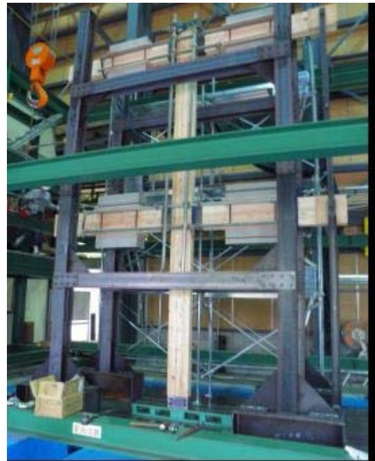
Figure 3 : Test set-up of specimen on a shaking table.
