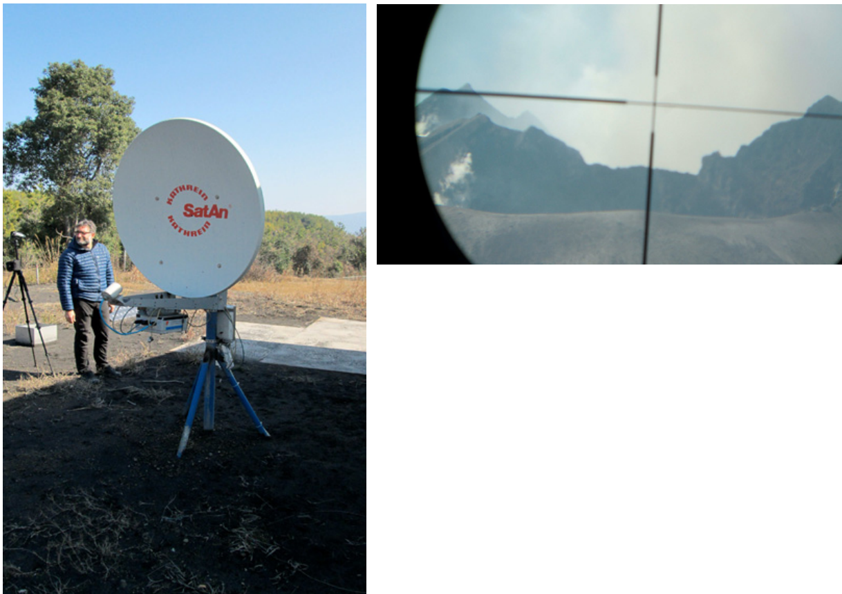
Figure 1. Left: Radar installed in the field. Top: Orientation of the radar beam above the rim of Minamidake crater. Opening of the radar beam is about 120 m at that distance.
