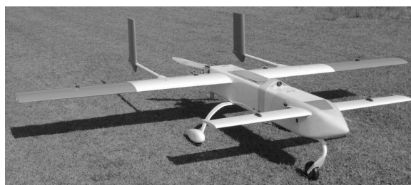
Fig. 3. Unmanned airplane "Phoenix-LR05" planned to use for aero-geomagnetic survey.
