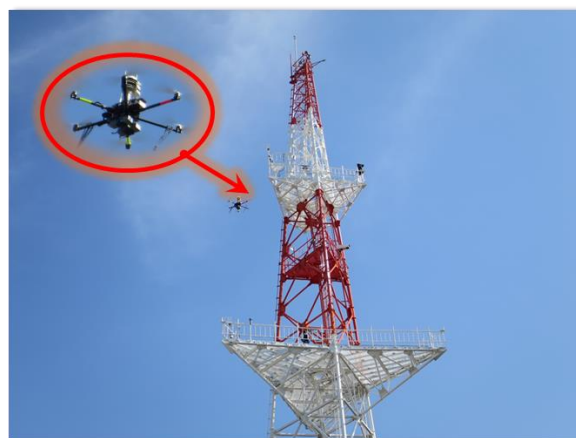
Fig. 2 Meteorological observation tower and hovering drone. Red circle shows zoom up image of hovering drone at 40 m height.
