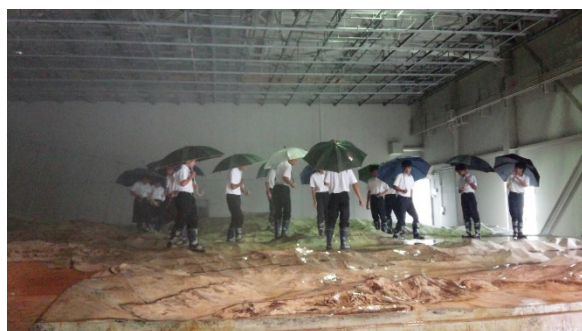
Fig. 1 Observation of the rain water flowing on the scale model of a river basin
