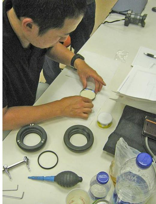
Photo 5: Adjustment of the alignment of objective lenses (Oct 2015)
