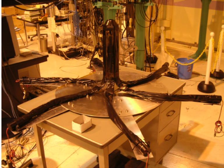
Figure 2.26: Picture of the combined six inner plastic scintillators.
