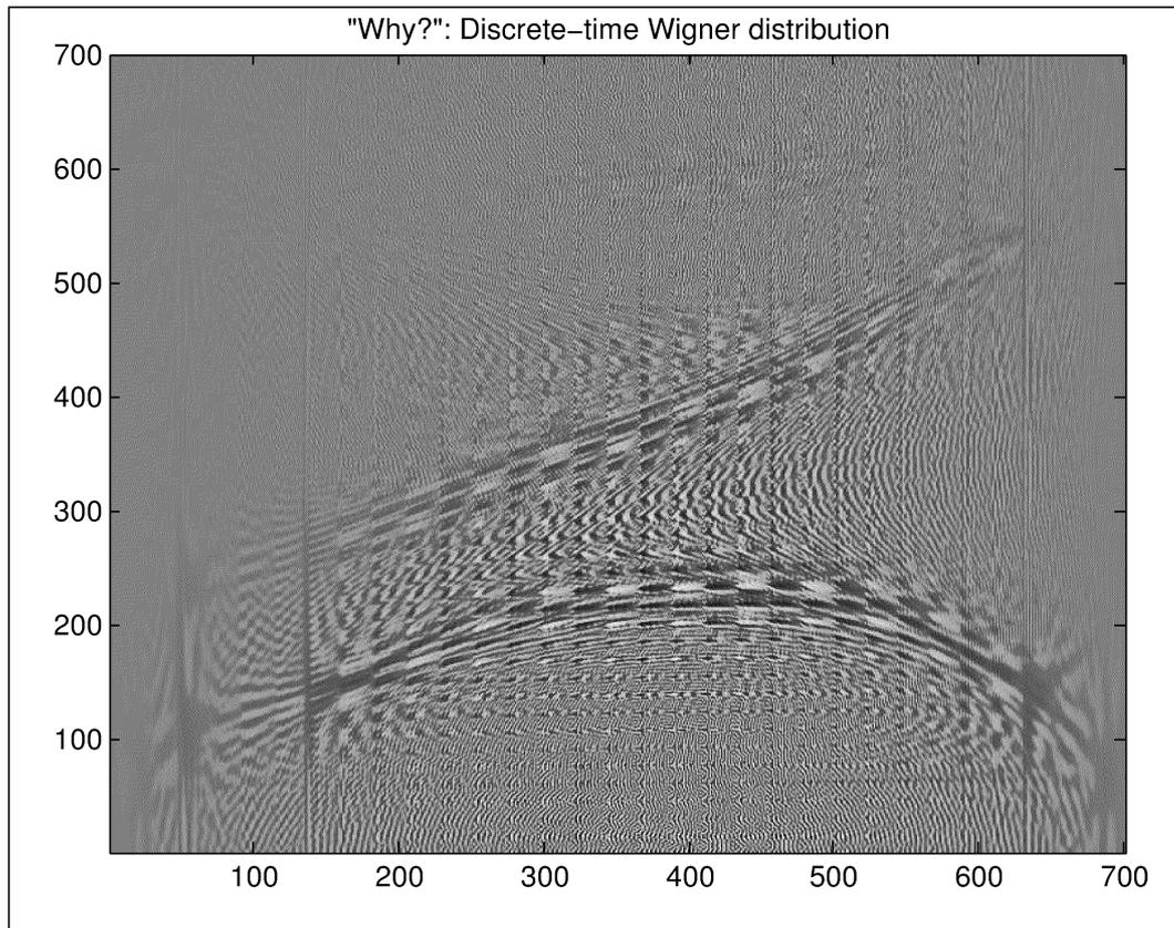
This illustrates how sensitive the Wigner distribution is to noise: the signal here was still rather well-behaving. To reduce the inherent interferences in the Wigner distribution, we are going to do smoothing by convolution. However, convolution of two Wigner distributions would lead back to the spectrograms, and we must eventually choose some other method:
