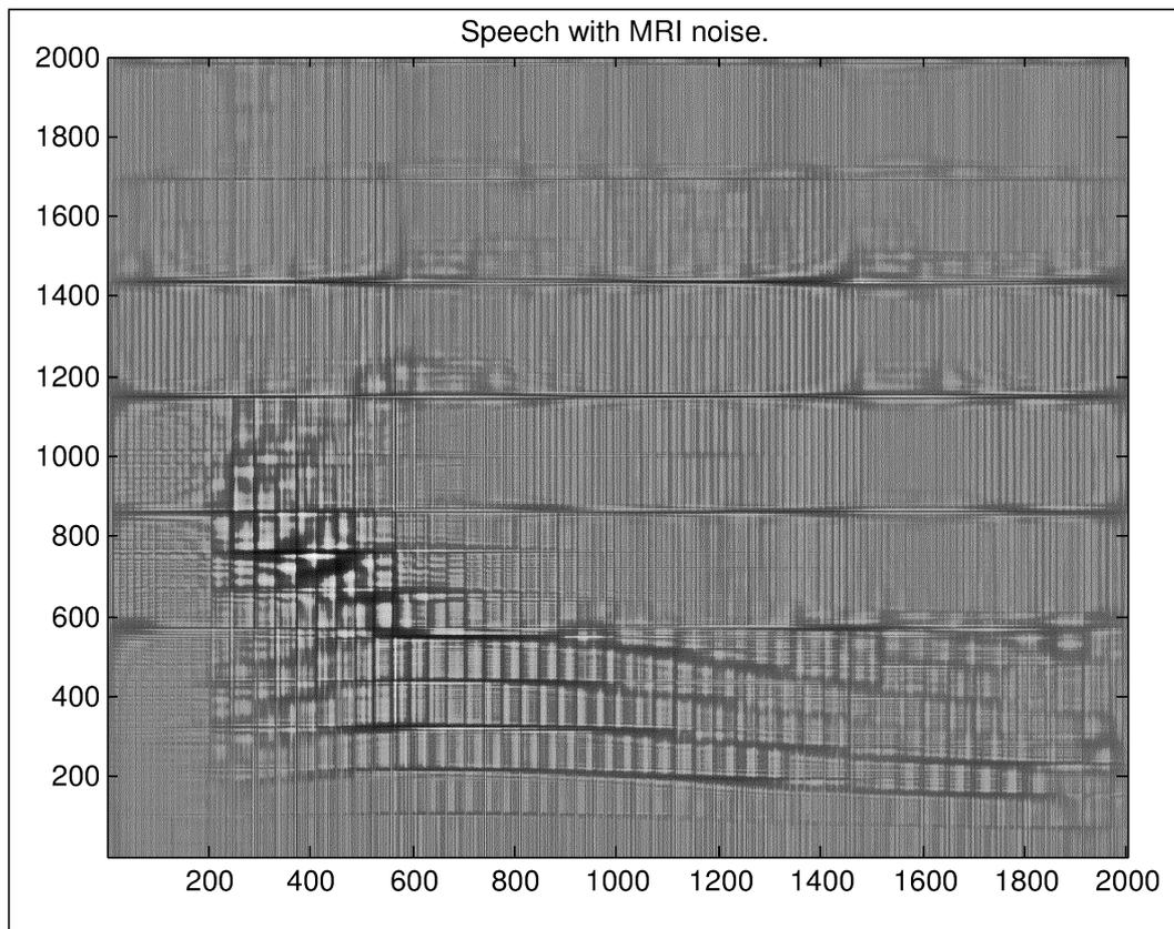
In the picture above, there are essentially two different grid-like patterns of rectangles of unit time-frequency area: the narrow and tall rectangles coming from the MRI, and the other rectangles coming from the speech. With this knowledge of time-frequency localization, it is possible to separate the speech from the MRI noise in a sharp fashion.
