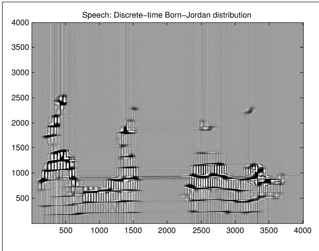
Of course, here the quality of the signal has suffered due to the heavy noise. For comparison, here is the Born-Jordan distribution of the original clean signal, without adding artificial noise:
