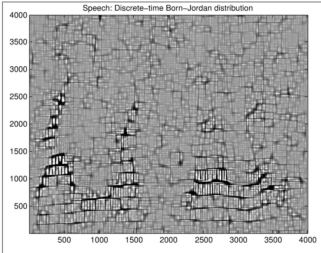
Then we apply two Born–Jordan localizations. In each of these localizations, the symbol is a characteristic function of a planar set, which is computed from simple natural conditions. These two simple conditions basically search those time-frequency regions where the energy density is “large-enough”. We obtain the enhanced filtered signal with the following Born–Jordan energy density:
