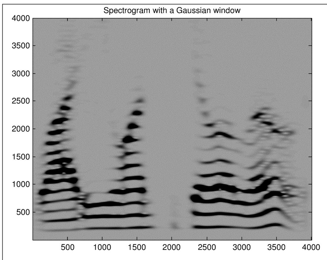
Moreover, we must remember that the choice of (a more-or-less arbitrary) time-analysis window in the Short-Time Fourier Transform heavily affects the shape of the spectrogram.
