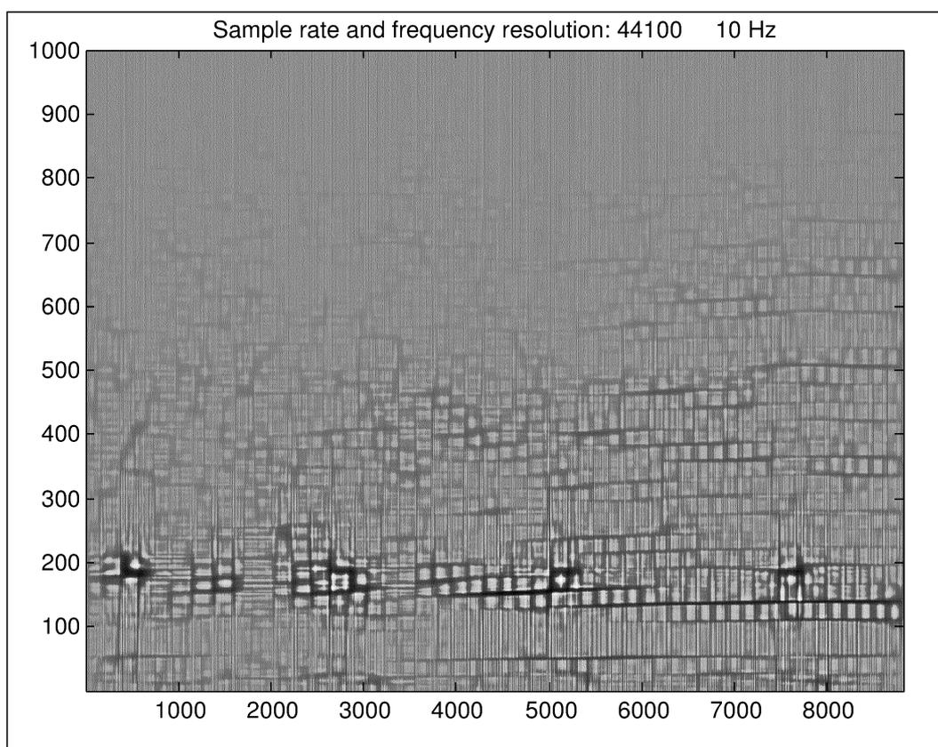
In such signals, there are simultaneously fast and slow spectral developments, which are rather troubling for spectrograms: Vertical features (snapping sounds, quick transients) would require very short time-analysis windows wiping out the horizontal features (whistling sounds), and vice versa.
