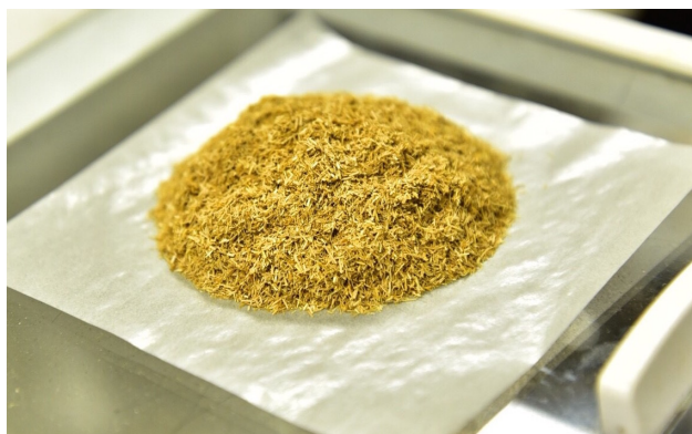
Figure 2.1 Rice straw sample with 150 \mu\text{m} – 425 \mu\text{m} of particle size
