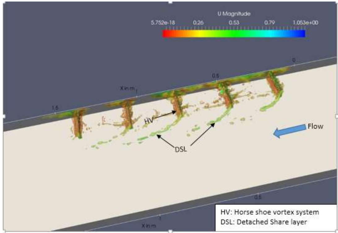
Fig.3.19 Visualization of the vortical structure of the mean flow using Q criterion of case 2.
