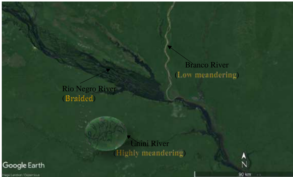
Fig.1.1 Satellite image of the Rio Negro, Branco and Unini River representing the different distinct planform of the river nearly in the same location (location: Manaus, Brazil, Oct 2018)
