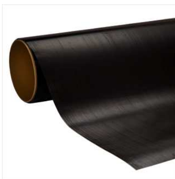
Figure 1-2. Image of a CFRP (TORAYCA®prepreg, TORAY, Japan) in which micrometer-scale-diameter carbon fibers are embedded in parallel in the matrix. 1
