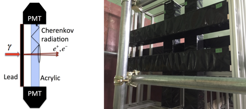
Figure 2.27: Left: Schematic view of a BHGC module (quoted from Ref. [73]). Right: a picture of BHGC viewed from downstream (quoted from Ref. [74]).
