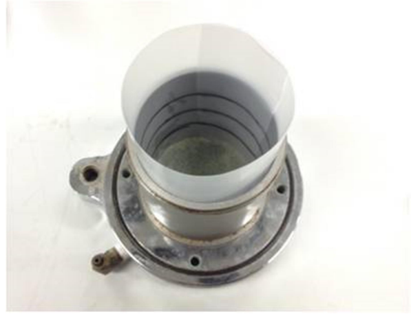
(b) mold with parafilm for compaction
