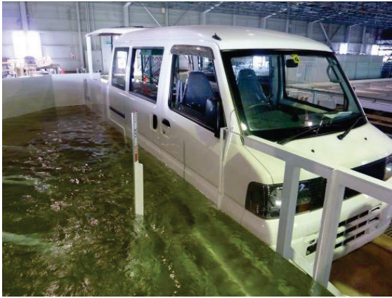
Photo 4 Experimental setup of car model (mini-vehicle).
