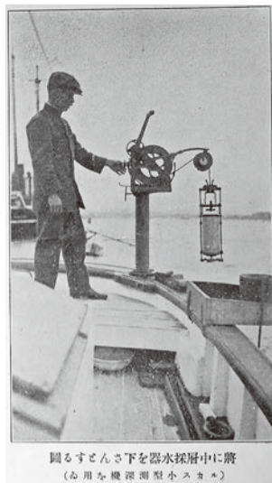
Figure 2. Kitahara Tasaku working with a Lucas sounding winch attached to a submersible intermediate-depth water sampler of his design (Kitahara 1921).
