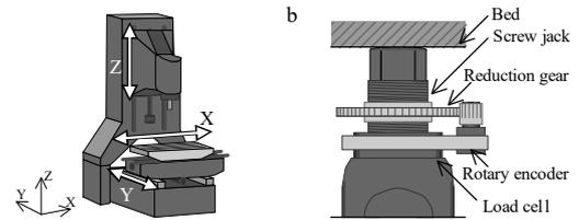
Fig. 2. Schematic of the machine tool: (a) Entire machine tool; (b) Jack bolt.
