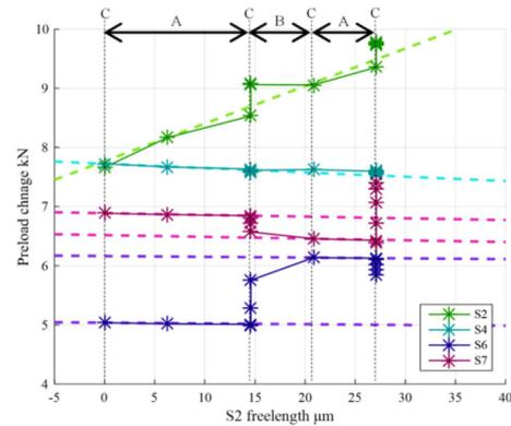
Fig. 5. Relationships between S<sub>2</sub> free length changes and preload changes of support S<sub>2</sub>, S<sub>4</sub>, S<sub>6</sub>, and S<sub>7</sub>.
