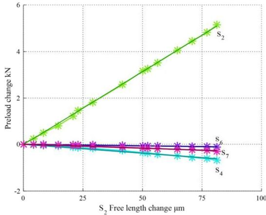
Fig. 4. Measured relationships between free length and preload changes in support S<sub>2</sub>; the slope of a regression line responds as a component of the stiffness matrix.
