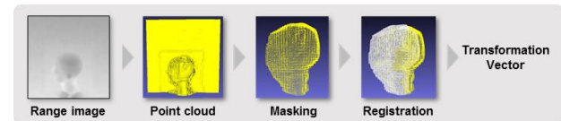
Fig. 2. Procedure of displacement estimation. Point cloud presented with white dots is corresponding to original position.
