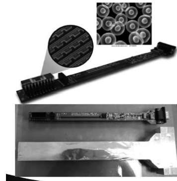
Fig. 1. Outline of silicon-on-insulator microdosimeter.
