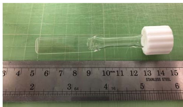
Fig. 1 A quartz cell with a Teflon cap. The thickness of the quartz windows was 0.5 mm, and the optical path was 1.0 mm
