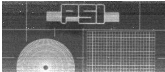
Fig. 2. Obtained neutron radiography of fine-structured Gd chart with nFPD. Integrating time was 5s at 1 MW operation. Fine patterns can be clearly observed.
